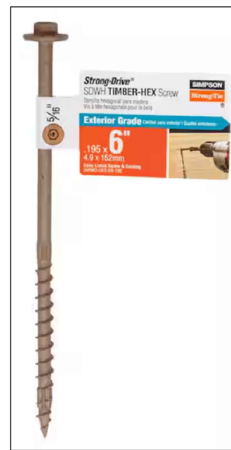
SDWH19600DB 0.195 IN. X 6 IN. 5/16 HEX. WASHER HEAD, STRONG-DRIVE SDWH TIMBER-HEX WOOD SCREW, DB COATING
